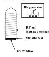
radios and power lines because a radio-frequency (RF) coil can act as an antenna.
